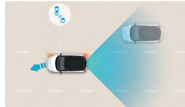
Blind Spot Collision Avoidance Assist (BCA): Radars detect traffic in the vehicle blind spot, warning drivers with an audible alarm when the indicator is used so you can be aware of the traffic around you. It will also take action itself, braking to help avoid a collision. Standard on Premium and Ultimate trims.
